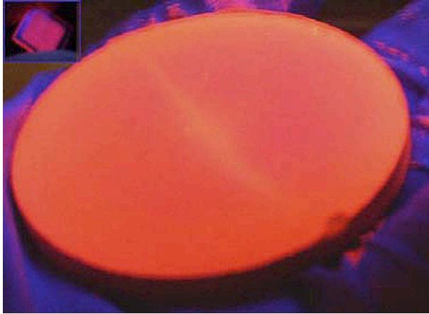
Fig. 2.5. Intrinsic luminescence of wide band gap BaCuSF.
